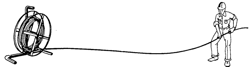
Fig. 15 Proper method of uncoiling wire rope for inspection.
